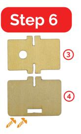
Following the picture below, start by attaching board 3 to the motor shaft. Then, use 7mm screws to secure board 4 to both board 2 and board 3.
