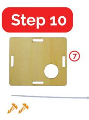
Start by using cable ties to organize the wires, then trim any excess ties with scissors. After that, secure board 7 using 7mm screws.
