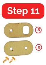
Attach board 8 and board 9 to the motor shaft using 7mm screws.
