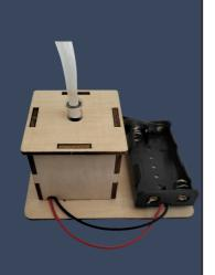
Install Board 5 by gently pressing it in the hole. Avoid using force. Take the battery and attach it with double-sided tape.
