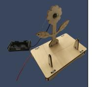
Your resistance wire will look like a spiral. Tie one end of the resistance wire to a nut. Guide the resistance wire through the round holes in Board 4 and 5. Finally, connect the other end of the resistance wire to another copper piece on the lamp holder.
