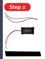
Refer to the circuit wiring diagram in STEP 1, First put the heat shrink tube on the red wire and then connect the wire cores together, then completely cover the wire core with the heat shrink tube, bake the heat shrink tube with a lighter to make it shrink.
