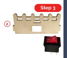
Refer to the picture below, install the ship type switch on plate 2.
