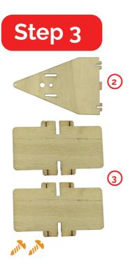
Put the two number 3 boards on top of board 2 and use two 7mm screws to attach them at the bottom.
