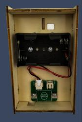
Install the battery box inside the lamp base using 4mm screws. Then, put the batteries into the battery box.
