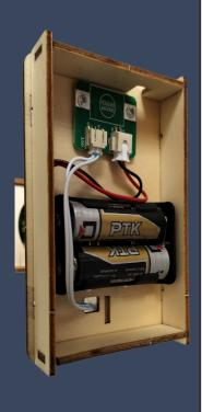
Insert the other end of the terminal wire from the LED module into the 2.0 connector on the switchboard.
