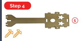
Install board 5 on top of boards 4 and 6 and secure it using 4mm screws.
