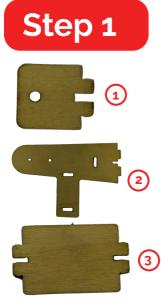
Use 4mm screws to install two board 1's on board 2, and then use 4mm screws to install board 3.
