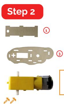
Use 2 x 7mm screws to attach board 1 to board 3
