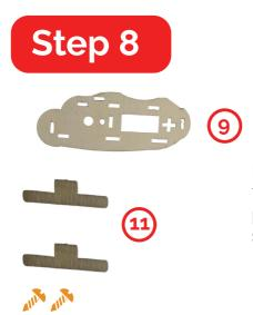
First, attach the no 9 board with 7mm screws. Also, add two no 11 pads. Do the same for the other side.
