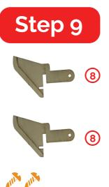
Insert two no 8 boards into board 2. Make sure they fit in tightly. Screw them in place using two 7mm screws.
