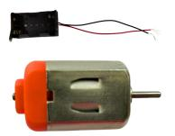
Pass the ends of the red and black wires from the battery box through the copper tags of the motor. Wrap them tightly around. Connect the red wire to the left and the black wire to the right.
